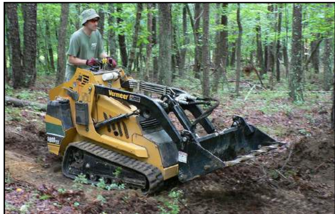
Pathfinders has received grants and donations that have allowed purchase of a mini-skid steer to assist with trail building.
